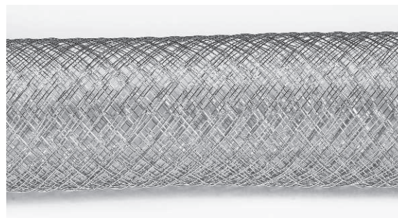
Figure 1 ♦ Close-up view of the multiple layers of cobalt alloy wires comprising the Cardiatis Multilayer Flow Modulator.
